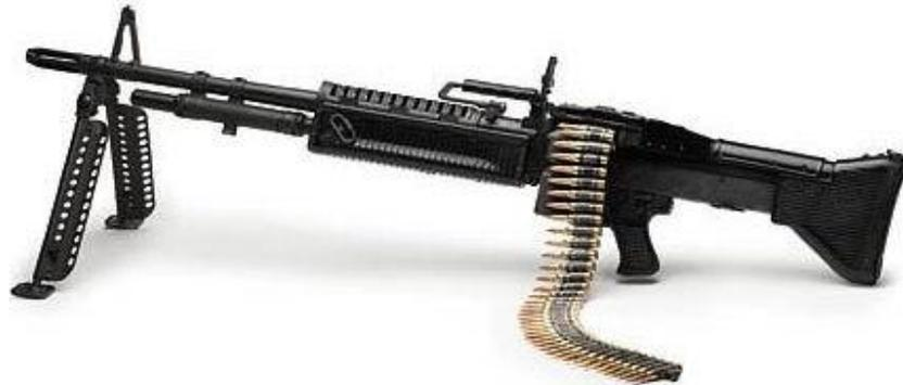
**The M-60 machine gun was a belt fed, gas operated, full automatic, gun which fired a .308 caliber or 7.62 mm cartridge.**
