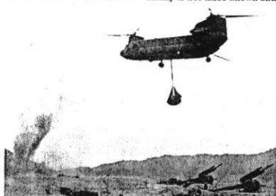
A CH-47 Chinook lowers a sling load of ammo for 155mm howitzers as the helicopters are busy hauling in the supplies necessary to build an instant LZ.
