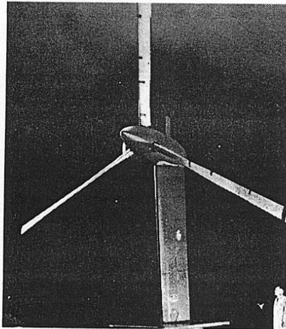
The blades of a 25-foot diameter aircraft propeller stand motionless after breezing through tests in a wind tunnel at a simulated speed of 408 knots. The propeller is being considered for use both during vertical take-offs and forward flight. The National Aeronautical and Space Administration and the U.S. Army Research Center, Moffett Field, Calif. (Photo courtesy Bell Helicopter Co.)
